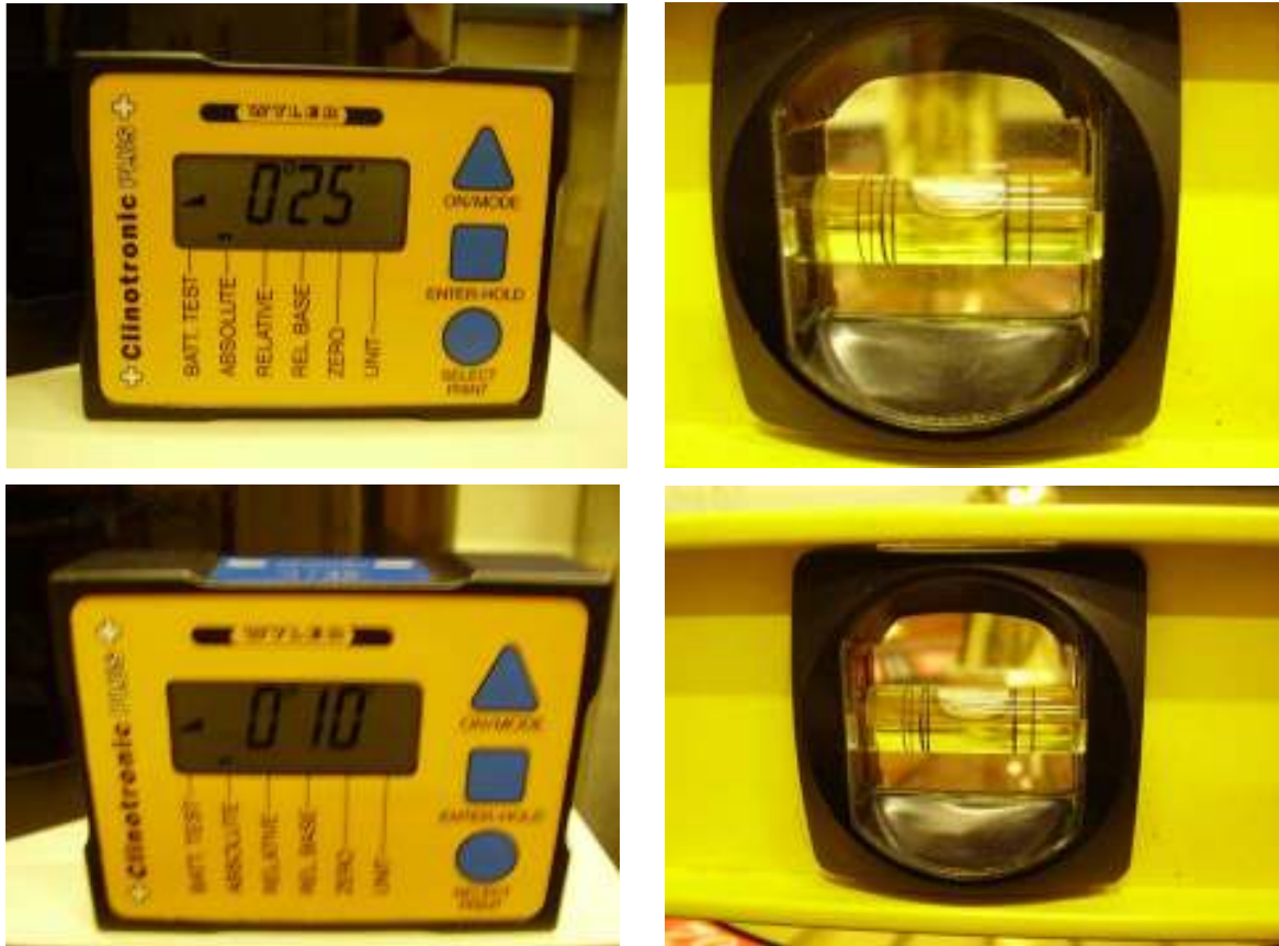
Figure 1 – Comparison of inclinometer and spirit level
